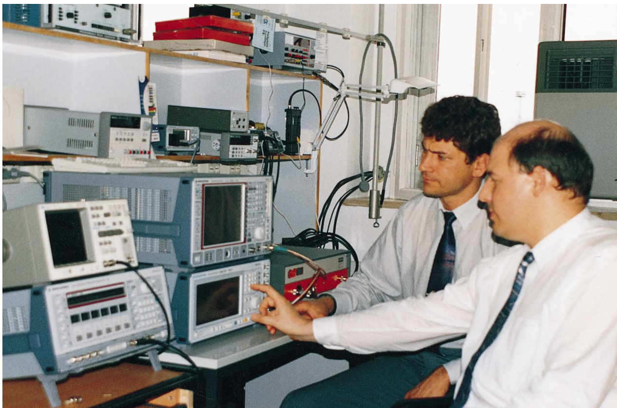
FIG 1 Test setup for generation of Inmarsat-E distress call data at Berlin-based company navtec Photo: Schäfer
