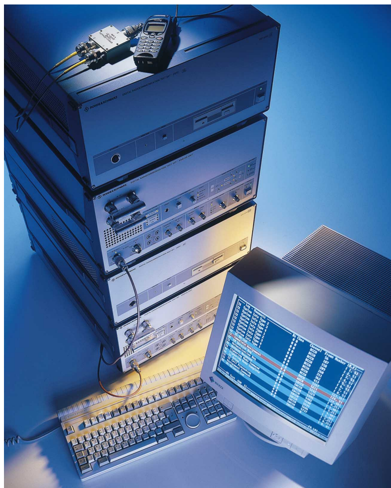
FIG 1 Multislot channel measurement of GSM mobile with DUO consisting of two Digital Radio- communication Test Sets CRTC Photo 43 250
